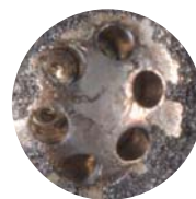
Injector after one P.i. treatment.
